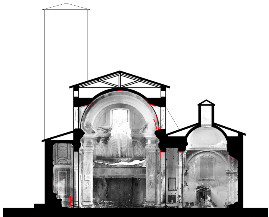
7. AA section of Saint Andrea church. Highlighted in red are cracks.
