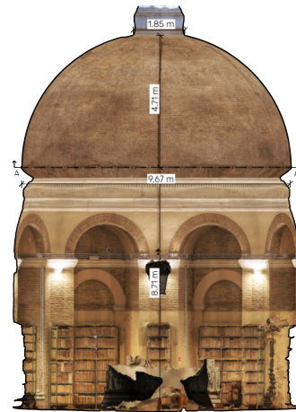
10a. Laser scan and photogrammetry surveys of the intrados Octagon San Basilio's dome in Vatican Basilica (Rome). Survey carried out by students of the Engineering Faculty of the University of Bergamo and SABE. Vertical section. Project by Antonio da Sangallo the Younger (around 1520).
